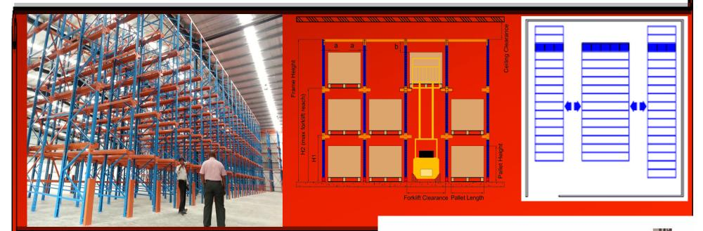
This kind of racking uses forklift to fetch goods. Space is more effectively used because the working passage for the truck and the storage space are combined together. For the character of first in - last out only one kind of goods can be stored along one working passage, or goods along one passage has to be done one at a time. It is widely used among business which goods are single species, normally use at wholesale, cold storage, tobacco and food industrial.
