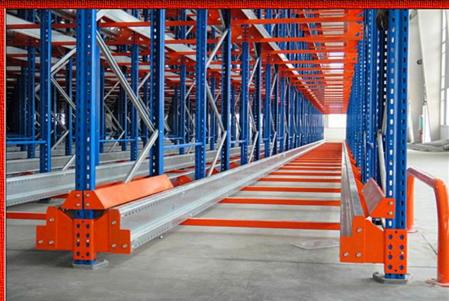
Shuttle rack system is a system composed of high density storage racking, shuttle and forklift. This new concept storage racking system is more powerful in operation than that of traditional storage racking, which enable it to take advantage of warehouse space sufficiently. The space utilization rate of it is more than 80%.
