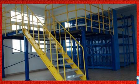
Mezzanine takes the multi-tier rack structure. It can be designed into multi- -floor (usually 2-3 layer), with stairs, handrails and cargo lift, etc.. Floor panel usually used cold-rolled steel floor with mutual buckle type structure. It can be equipped with lighting system. The load capacity of each level shelf is usually within 500 kg,; while the loading of floor panel is between 300-1000kgs per square meter.
