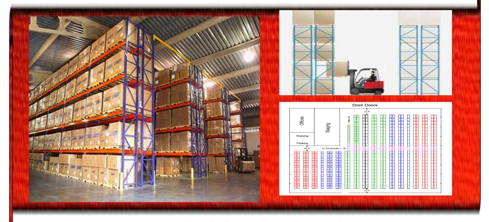
Pallet racking can be adjustable and suitable for the forklift working. There are two kinds of aisle can be chosen one is normal aisle about 3000mm; another aisle about 1700mm which require special forklift to fetch.
