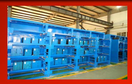
Mold Storage Rack is mainly used for storage of all kinds of mold such as plastic mold, metal molds, casting mold, powder metallurgy mold and extrusion die.
