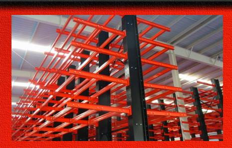
This type of racking is suitable for keeping materials of big, long size, such as pipes and shaped steel, etc. Materials are put on the cantilever. Forklift truck and stacking crane are often applied with the rack. This is suitable for small warehouse and popular with machinery processing and building – material supermarket.
