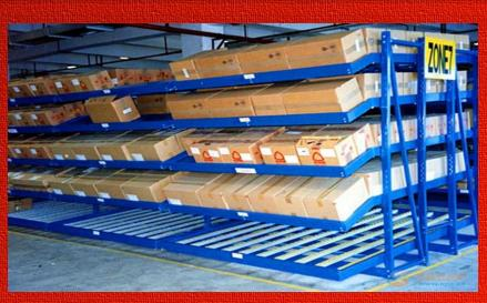
Depending on gravity, goods stored on carton flow racking can move automatically, which can realize "First In First Out" operation. It is suitable for storage of large quantity of similar goods. Both the efficiency of goods storage and picking and the space utilization rate are high.
